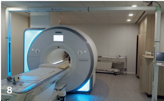
External laser bridge for MR treatment planning
