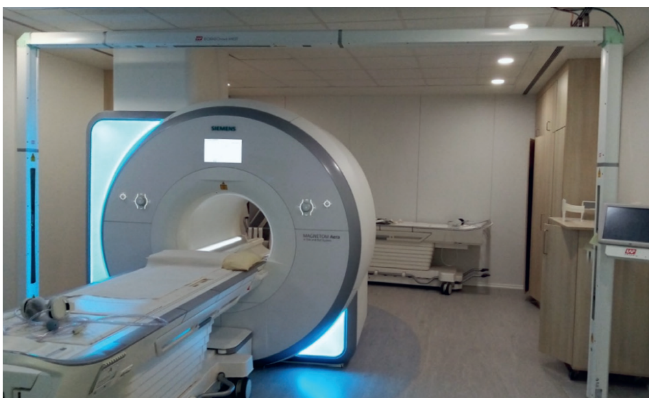
10 External laser bridge for MR treatment planning.
