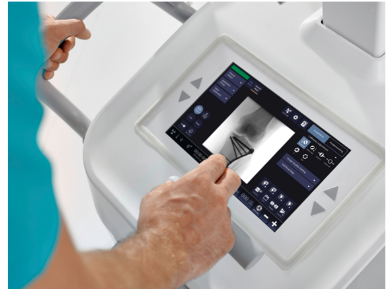
The smart touch user interface includes a feature for previewing acquired images.
