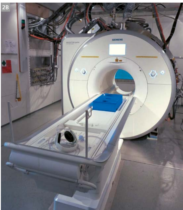
2 1.5 Tesla demonstrator during magnet testing and MRI system testing in 2014. (2A) Magnet tests in Oxford. (2B) System tests in Erlangen.
