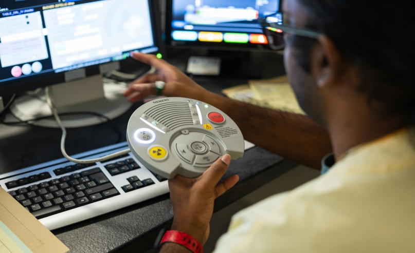
This device is used to communicate with the patient, move the patient bed, and start the radiation of the CT.
