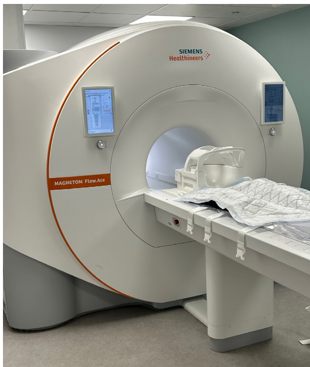
1 The 1.5T MAGNETOM Flow.Ace at Lumbry Park. Thanks to the DryCool technology, the system has no quench pipe and an ultra-compact footprint of only 24 m 2 .
