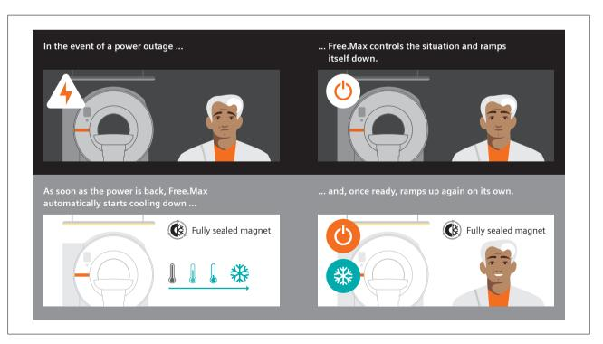
4 Always on the safe side: Intelligent automated ramp-down feature acts faster and smarter than any human could in the event of loss of refrigeration.
