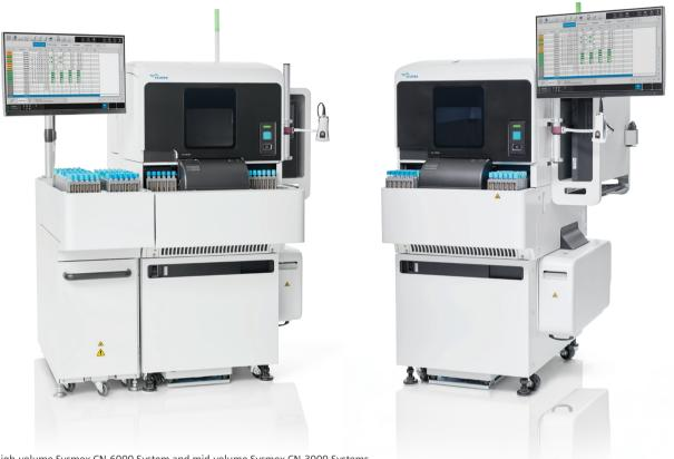
The high-volume Sysmex CN-6000 System and mid-volume Sysmex CN-3000 Systems are both available with the optional sample handler shown above on the left.
