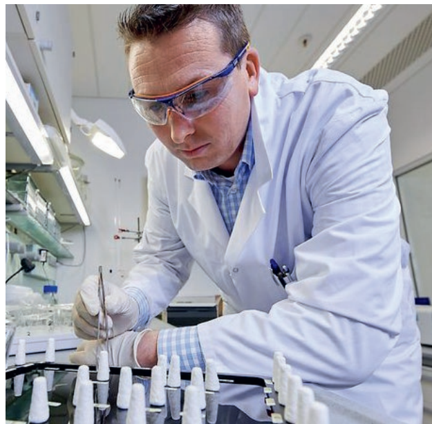
4 Sebastian Köppl testing a display for its resistance to cleaning agents and disinfectants.
