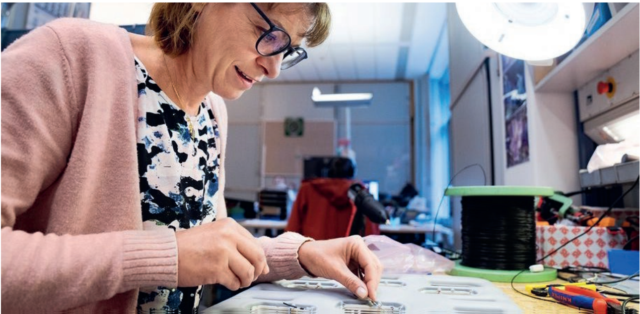
2 Yvonne Candidus wires the antennas for the local coils.
