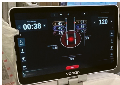
Real-time procedural feedback from thermocouples as shown on the IntelliBlate System interface
